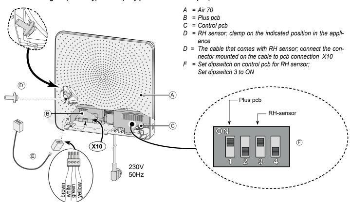
If the RH sensor (humidity sensor) measures an increase of the RH for a number of minutes, the ventilation capacity is automatically increased to ventilation mode 5.
